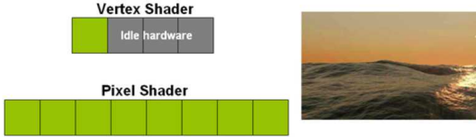
Figure 4: Utilization of pipeline GPU on fragment-intensive workload.
